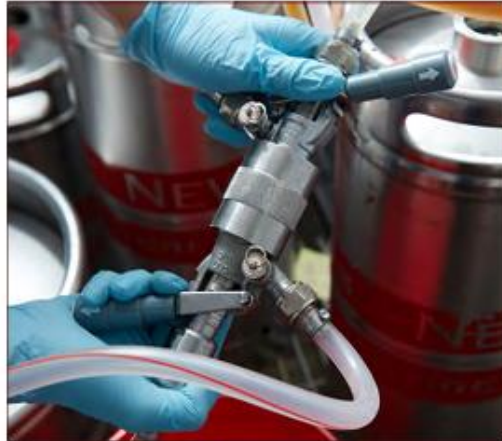
Figure 7.12. Couplers can be linked to aid in recirculation cleaning.
